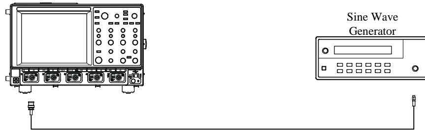
Figure 5-4 : 50Ω Bandwidth Equipment Setup
